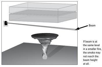
Figures 5, 6, 7. Pre-stratification and detector placement
