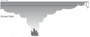
Figure 4. Typical smoke field in the shape of an inverted cone
