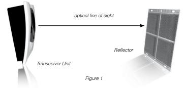
Beam smoke detectors operate on the principle of obscuration. As a smoke field develops, the detector senses the cumulative obscuration – the percentage of light blockage created by a combination of smoke density and the linear distance of the smoke field across the projected light beam. The threshold is typically set by the manufacturer to match the conditions of the installation.
