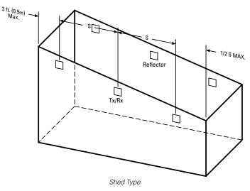
Figures 10 and 11. Mounting on Sloped Ceilings
